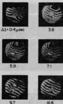
FIG. 5. Interferograms of the Scylla IV discharge corresponding to the current waveform of Fig. 4 with an initial deuterium pressure of 15 mTorr. A few of the 56 photographs taken by the framing camera are shown for illustration and identified by the time  $\Delta t$  after application of the primary bank. Exposure time per frame: 0.42  $\mu$ sec.
