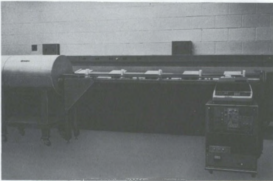
FIG. 7. Passive neutron-coincidence counter for measuring ^{240}\text{Pu} content in FBR-type fuel pins. The system includes ^3\text{He} thermal-neutron detector, automated fuel pin loader and translator, and electronics and data control rack.
