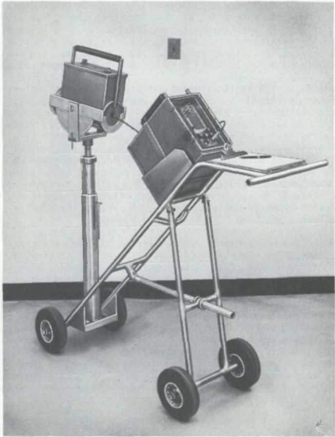
FIG. 10. Cooled, portable NaI gamma spectrometer for assay of ^{235}\text{U} inside an operating gaseous-diffusion plant.
