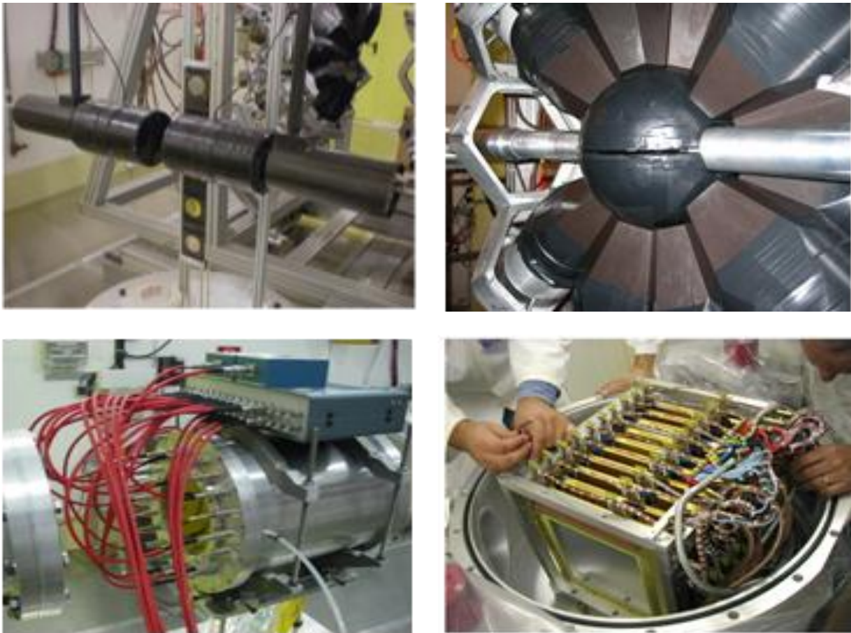
FIG.1. Photographs of the detectors mentioned in section 2. Top-left: C_6D_6 . Top-right: TAC. Bottom-left: MGAS. Bottom-right: PPAC.
