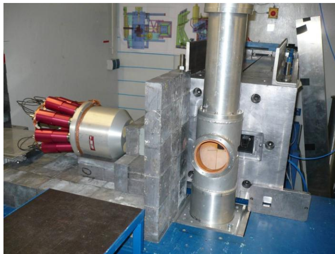
FIG. 2. The PGAA facility at Garching without the lead shielding. To the left: the BGO with the collimator and the frontal lead shielding, in the middle: the sample chamber (lined with ^6\text{Li} -containing polymer), behind it the end of the neutron guide and its shielding.
