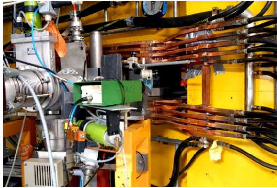
FIG. 2. The neutron production area at the QMN facility: the incoming beam line (to the left, in the foreground), the bending magnet (in the background), and the target elevator (upstream the magnet).
