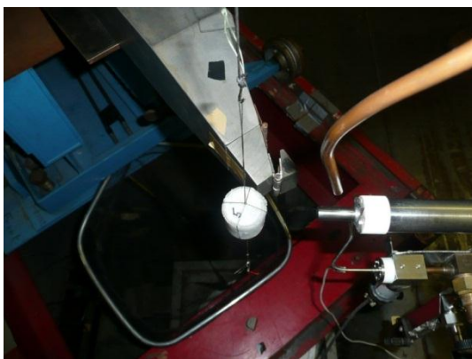
FIG. 2. Top-down view of the end of the neutron TOF beam line. The accelerated charged-particle beam enters from the right and produces neutrons in the 3-cm long gas cell at the end of the beam line. The tungsten shadow bar prevents the detector from directly viewing the gas cell.
