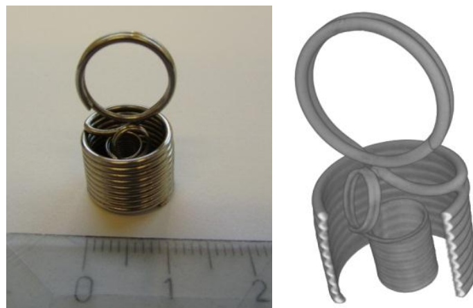
FIG. 3. Tomography picture of two springs clearly shows the internal small spring placed inside the bigger one.
