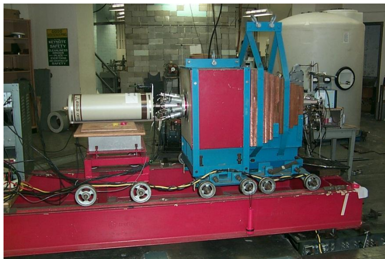
FIG. 8. Singles γ ray measurement configuration. The carriage is shown at 90° to the beam direction.
