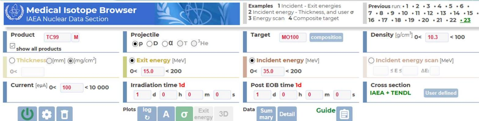
• Effective target thickness : 0.161 cm • # incident particles: 6.24151E+14 [s<sup>-1</sup>] • Produced heat in target : 2.000 kW • Activities less than 1.0E-9 GBq are not displayed
