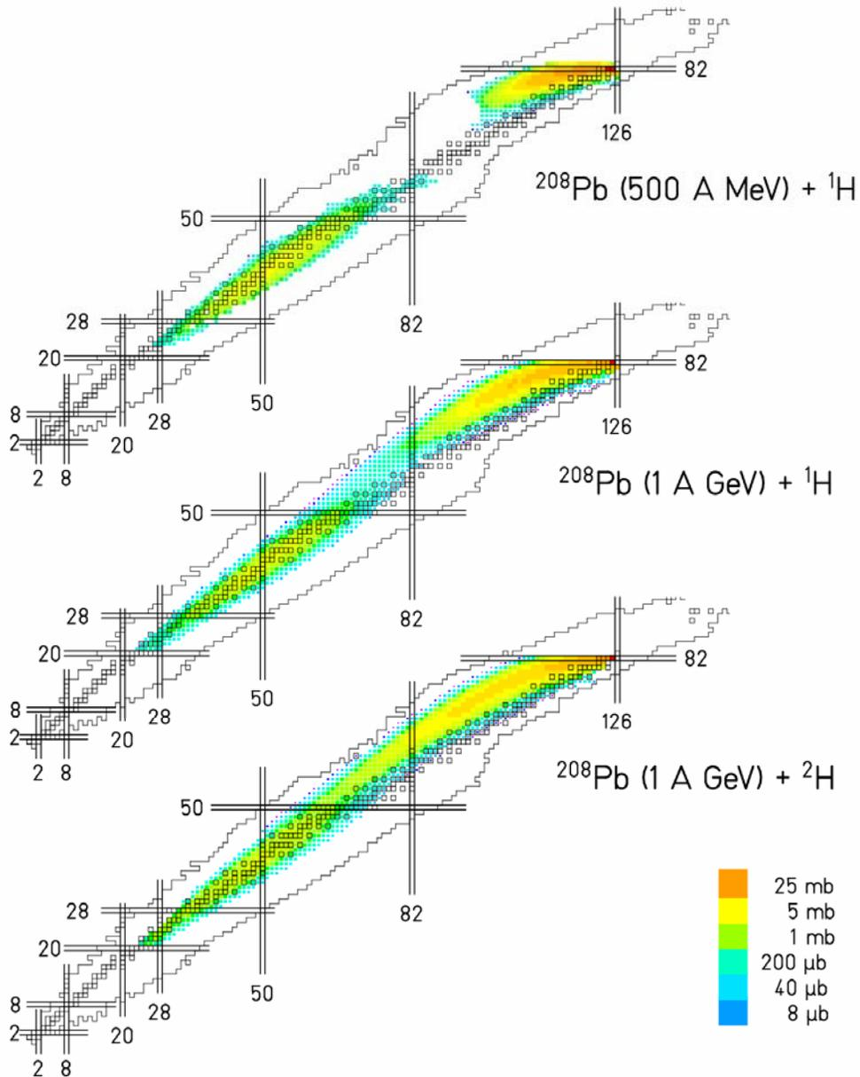
Increase of beam energy leads to higher excitation energies after INC and to larger mass loss in evaporation.
