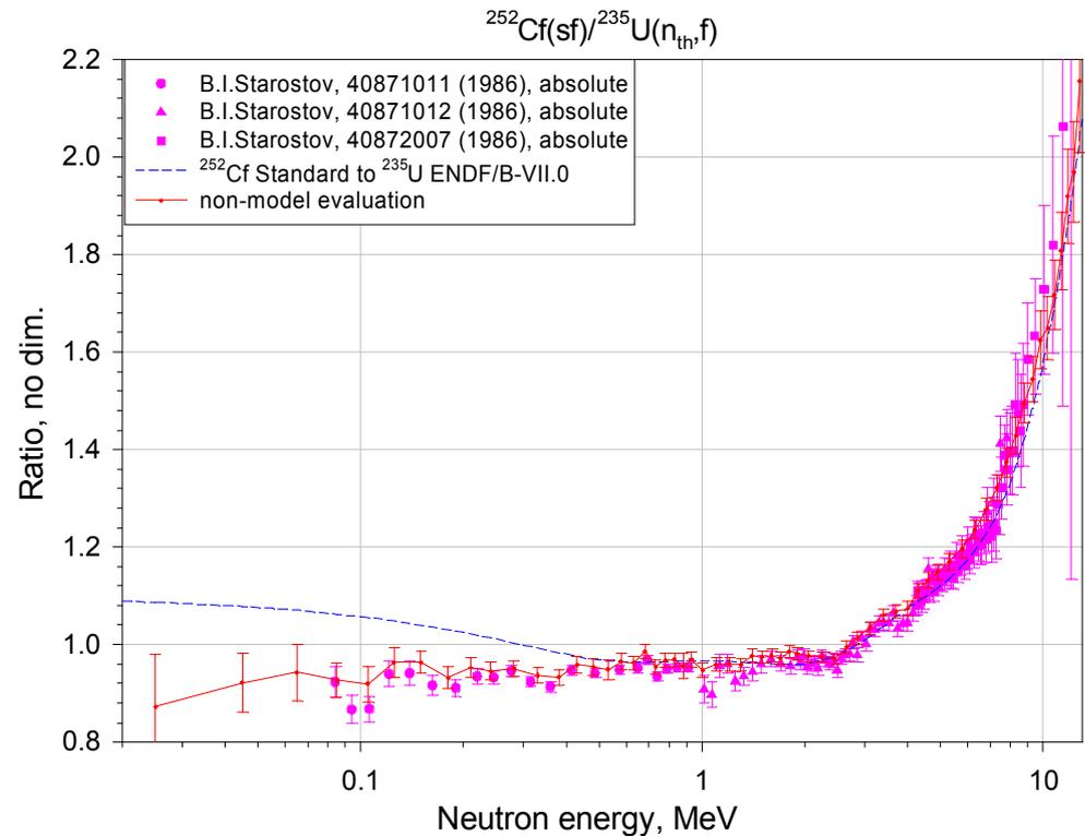
Comparison of the results of measurements of absolute ratio of the PFNS spectra  $^{252}\text{Cf}(\text{sf})/^{235}\text{U}(\text{n}_{\text{th}},\text{f})$  in linear and logarithmic scales on neutron energy.
