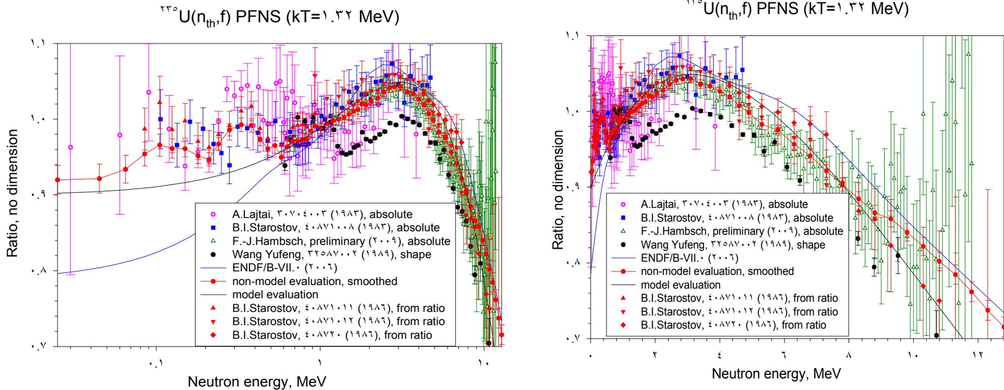
Comparison of the  $^{235}\text{U}(n_{\text{th}}, f)$  PFNS in linear and logarithmic scale on the neutron energy.
