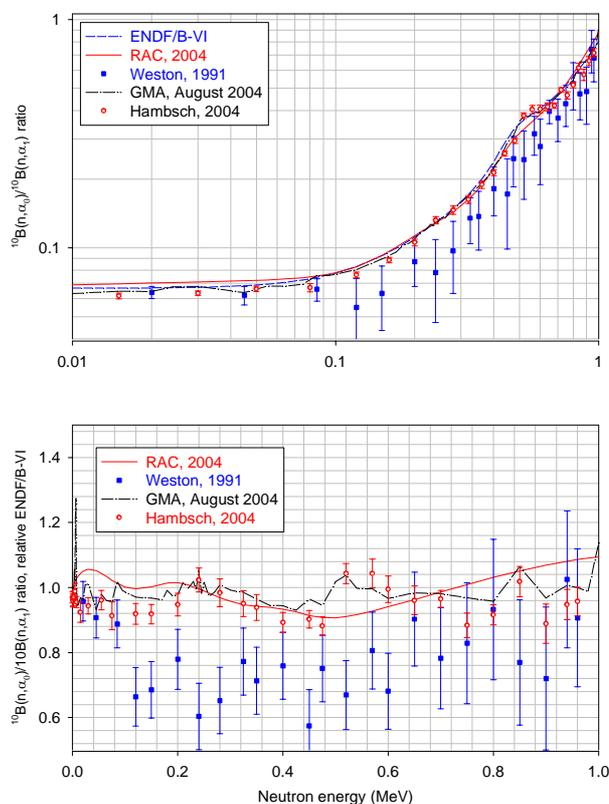
**FIGURE 7.** Comparison of measurements and calculated results from various evaluations for the  $^{10}\text{B}(n, \alpha)$  branching ratio.
