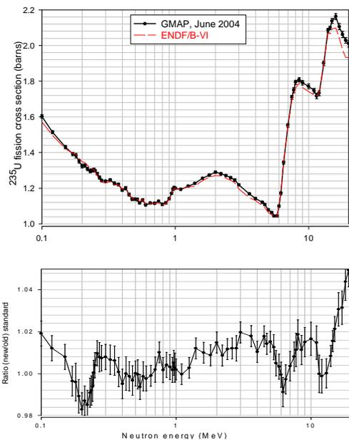
**FIGURE 6.** Comparison of old and preliminary new standards for the  $^{235}\text{U}(n, f)$  cross section.
